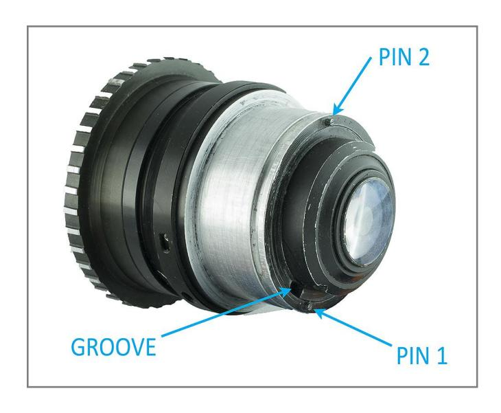
2) Apply the lens onto the adapter. Push the lens inside the adapter (do not use much force) up to resistance. Make sure that the "ADAPTER PIN" is lined up with "GROOVE" and the "SECURE SCREW" is loosen. Then give the lens push. You should hear a "click" sound.
